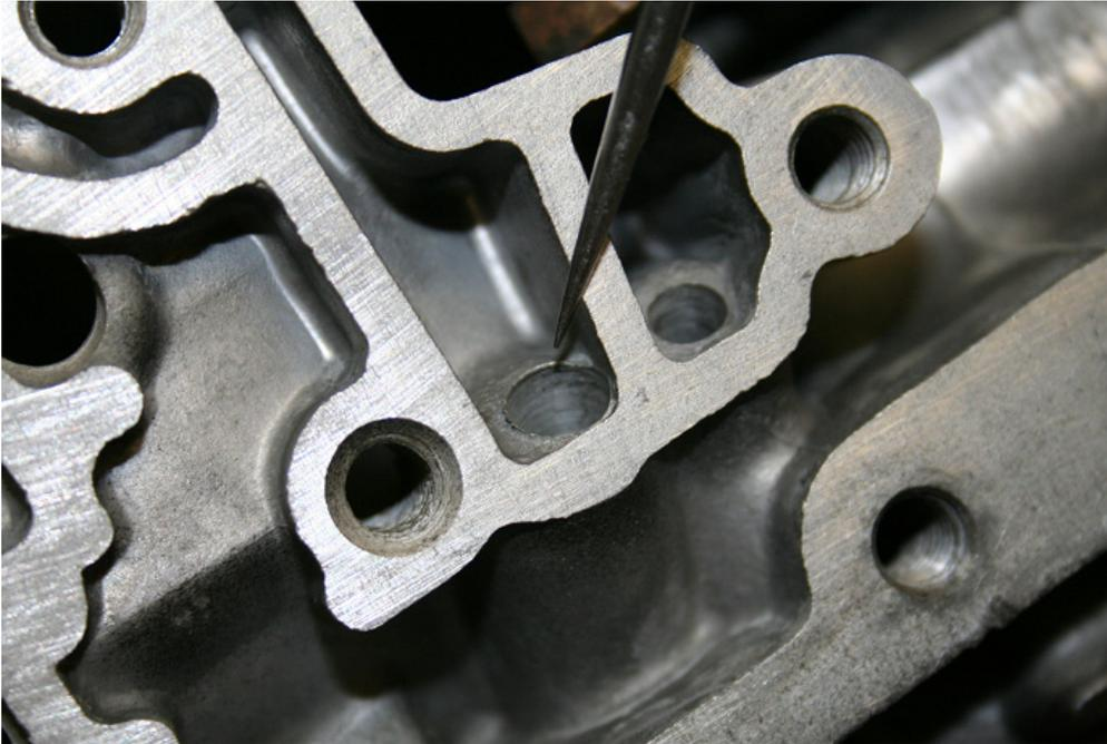
5. Install band servo plug (steel) as shown below.
