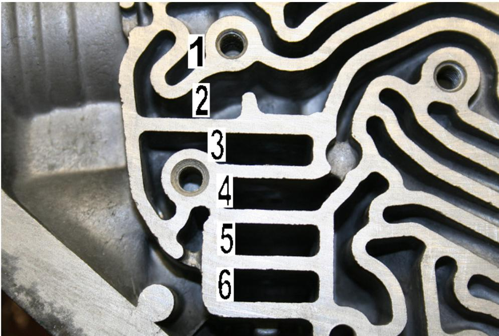
Brake ON: Lands 3 & 4 are connected. Brake OFF: Lands 4 & 5 are connected.
