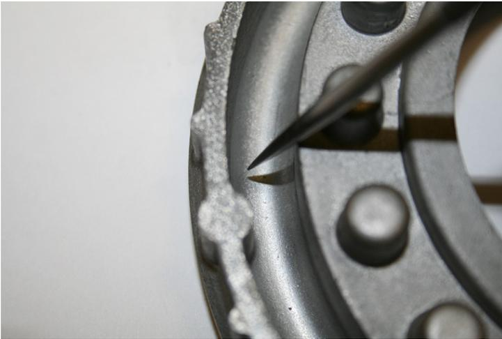
4. Reassemble drum with new lip seals on piston. Discard center seal from drum. Set clutch clearance at .045-.055". Install 17 included new return springs.
